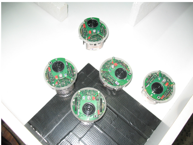
Fig. 5 e-puck robots in a collective robotics application
