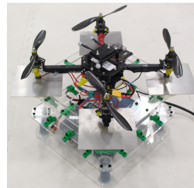
Fig. 5: Quadrotor resting on charging station.
